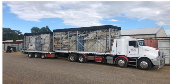
6.0m "high" cage on trailer with 8.0m cage on truck
